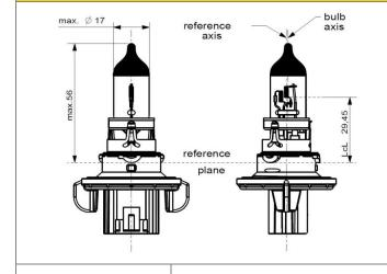
Light center length: 29,45mm Bulb diameter: max. 17mm
